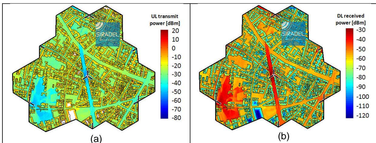
**Figure 2: Example of (a) UL transmit power ground-floor map and (b) DL received power ground-floor map.**
